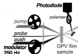
**Figure 4.** Schematic image of pump-push-probe experiment.
