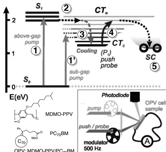
**Figure 2.** Schematic image of pump-push experiment.
