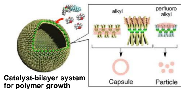
Fig. 3 Polymer assembly in a synthetic catalyst-bilayer system made of pentasubstituted [60]fullerene anions.
