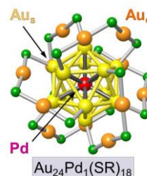
Fig. 3 A proposed structure of \text{Au}_{24}\text{Pd}_1(\text{SR})_{18} with Pd@Au 12 core.
