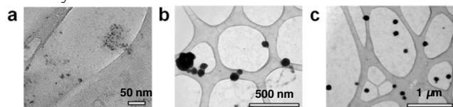
*Fig. 6* CdTe/CytC SPs in the course of the assembly 3 hrs (a), 24 hrs (b), and 72 hrs (c).
