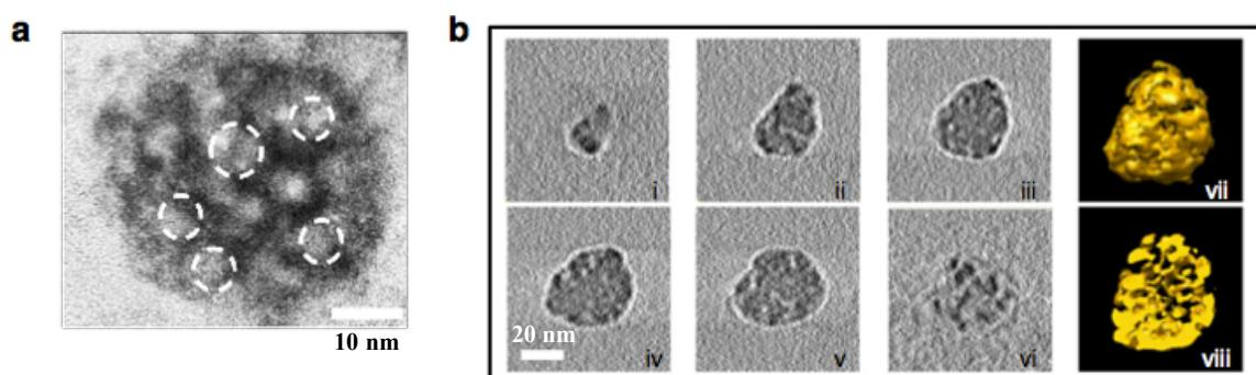
*Fig. 3* (a) High-resolution TEM (HR-TEM) image of the SP. (b) TEM tomographic reconstructions of CdTe / CytC SP: X-Y slices (i-vi) of the SP, shown in every 4.8 nm through the volume. 3D surface rendering(vii) and cross-section (viii) of the SP.
