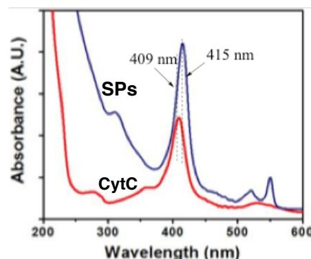
*Fig. 4* UV-Vis spectra of CytC and SPs.
