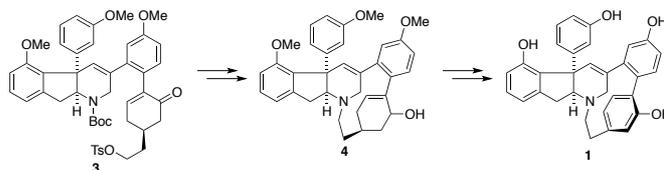
**Scheme 2.** Mechanism of the proposed oxidative phenol coupling toward *p*-cyclophane moiety.
