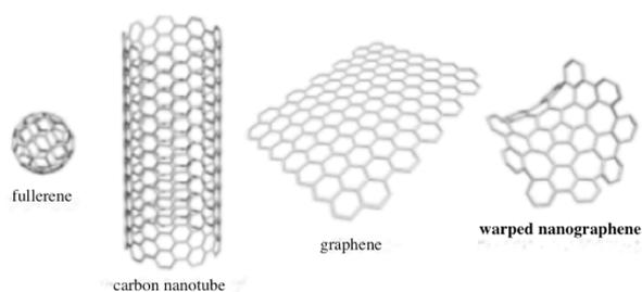
**Figure 1.** The structure of nanocarbon
