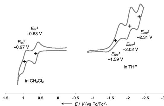
**Fig S12.** Cyclic voltammogram of  $(t\text{-Bu})_{10}\text{C}_{50}\text{H}_{30}$  (**8**) in  $\text{CH}_2\text{Cl}_2$  (1.0 mM) and THF (1.0 mM). Scan rate:  $100 \text{ mV s}^{-1}$ ; working electrode: Pt; reference electrode:  $\text{Ag}/\text{AgNO}_3$ ; electrolyte:  $n\text{Bu}_4\text{NPF}_6$ .  $\text{Fc}/\text{Fc}^+$  = ferrocene/ferrocenium.
