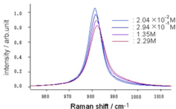
**Fig. 2** Concentration dependence of the  $\text{SO}_4$  symmetric stretch Raman band of magnesium sulfate in water.
